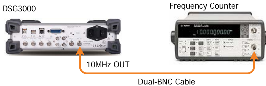
Figure 2-1 10 MHz Reference Output Accuracy Test Connection Diagram
