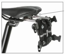
**ONE** Attach the bracket to your saddle rails. See steps 1 thru 3 on page one.
