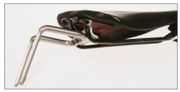
Final assembly complete. Although the 2311 back plate is hardened aluminum (T-6), it will still bend. This is normal and this "giving" will dampen some of the vibration or shocks to the bag system.
