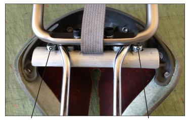
STEP 3A—EXTRA BOLTS Once you have assembled everything, forcefully grab the bracket and attempt to move it up and down. If you find that your bracket does slide upwards & you have room for an extra pair of bolts on the outside of the rails, we recommend this step.
