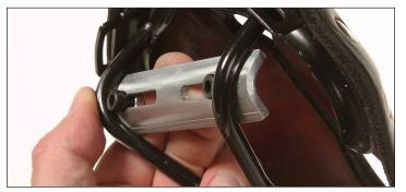
**STEP 2** The plate should be near the center of the curve of the rails.
