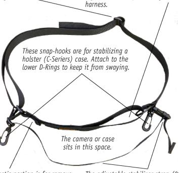
The small Velcro/elastic portion is for removaing the front strap as the front portion is optional when used with a holster case. The adjustable stabilizer strap (20mm / 3/4" wide) goes around the camera lens or body. A quick-release buckle makes accessing your camera a cinch.
