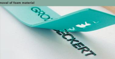
Now the 3-D image is available. An acceptable result is only achieved with precise stitching. Thread is covering the foam material without gaps and no stitches looped. The material must not be damaged and the 3-D-effect must be uniform.
