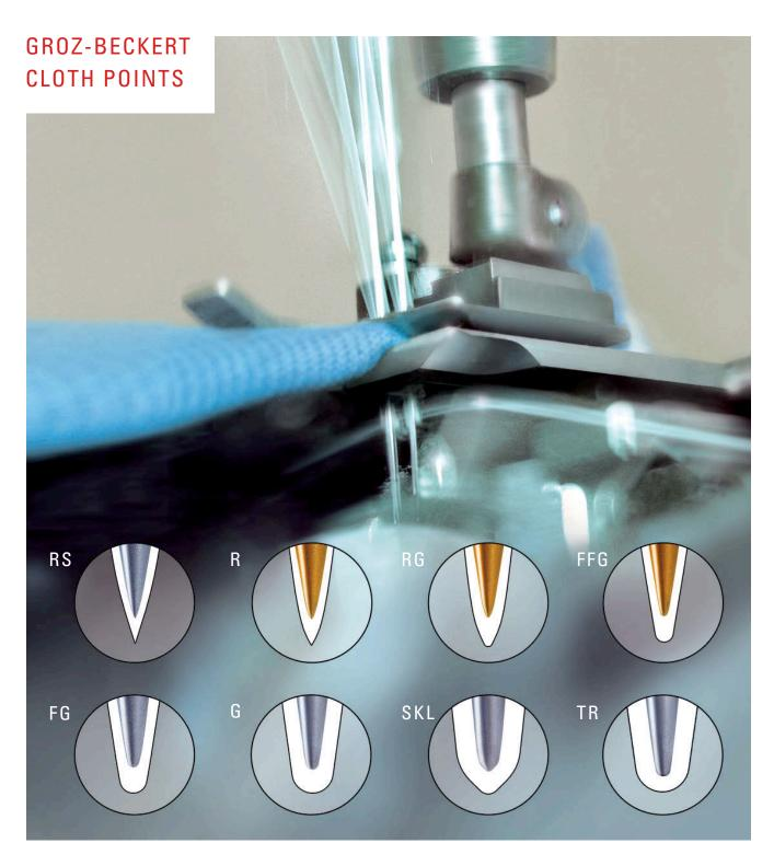
All textiles, whether woven, warped, felted or knitted, are sewn with a specific needle point shape to suit their structure.
