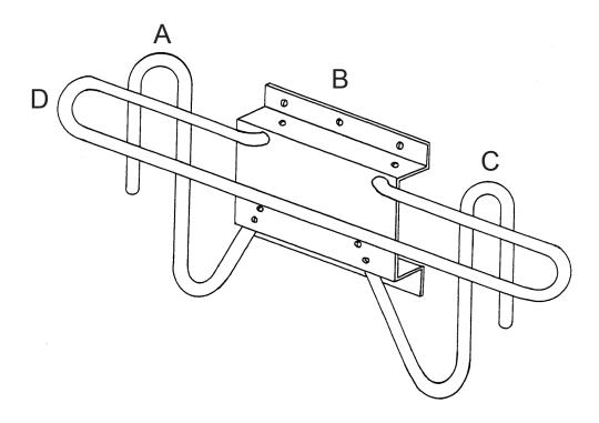
Insert glove holders (A and C) into holes on the bottom of the wall holder (B) and screw them in with the screws provided.
