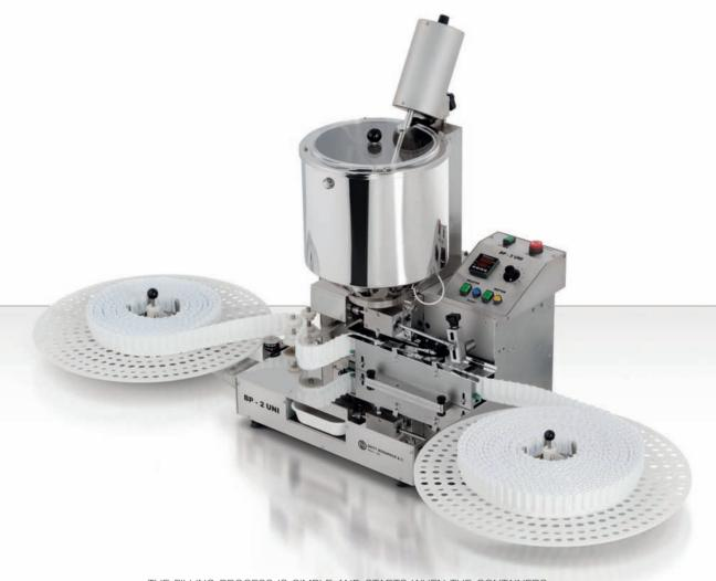
THE FILLING PROCESS IS SIMPLE AND STARTS WHEN THE CONTAINERS FROM THE LOADING DISC ARE AUTOMATICALLY UNWOUND AND FED UNDER THE DOSING NOZZLE, FILLED WITH MELTED SUPPOSITORY MASS WHICH IS KEPT AT A CONSTANT TEMPERATURE AND MIXED IN THE JACKETED HOPPER. THE FILLED CONTAINERS ARE AUTOMATICALLY REWOUND ON THE SUPPORTING DISC PLACED AT THE DISCHARGE OF THE FILLING MACHINE. IT IS COMPLETELY MANUFACTURED IN ITALY ACCORDING TO CE AND GMP RULES.
