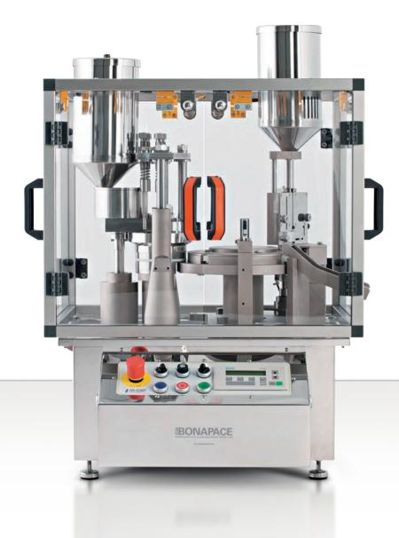
IN A FEW YEARS, THE IN-CAP XL HAS BECOME VERY POPULAR ALL OVER THE WORLD AMONG R&D LABORATORIES, PHARMACIES, HOSPITALS, ETC. FOR TRIALS RESEARCH, BATCH PRODUCTIONS, AND IN LABORATORIES FOR FULL PRODUCTION UTILIZATION. SUITABLE TO PROCESS POWDERS, PELLETS, LIQUIDS OR SEMI-SOLID PRODUCTS, TABLETS—MINITABLETS AND CAPSULES (CIC). THE MACHINE CAN BE SUPPLIED EITHER WITH TAMPING OR DOSATOR POWDER SYSTEM. IT IS COMPLETELY MANUFACTURED IN ITALY ACCORDING TO CE AND GMP RULES.
