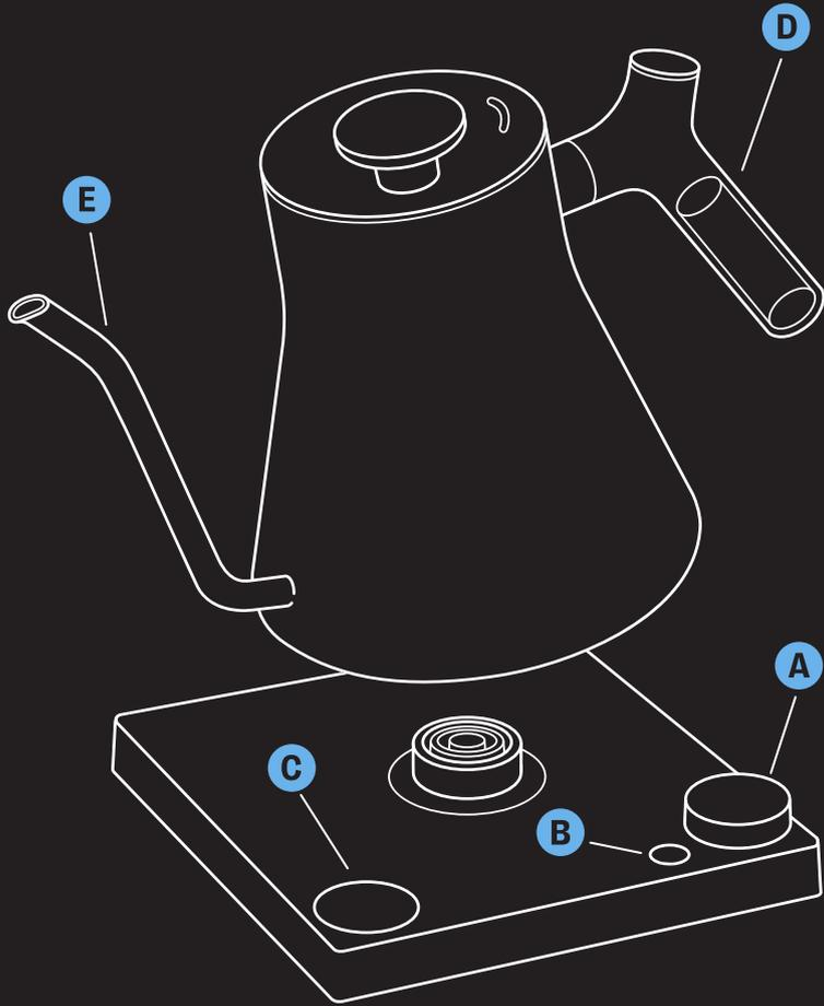
**A DIAL** One quick press to turn on the heat. One long press to start the Brew Stopwatch. Turn to select the temperature.
