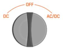
**LEFT POSITION:** All DC ports (12V DC sockets, Basecamp LED Light ports, and the USB ports) on, otherwise referred to as DC ONLY mode. This will also activate the LCD Display.
