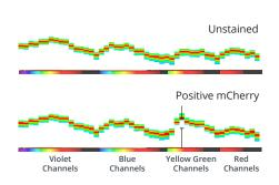
Spectrum plots of unstained and positive mCherry cells acquired on the Aurora. Note that the two spectra heavily overlap.
