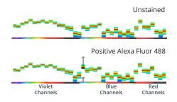
Spectrum plots of unstained and Alexa Fluor 488 stained cells acquired on the Aurora. Note that the two spectra heavily overlap.
