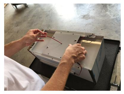
10. Now while sliding the inner kit into your outer shell, make sure the wires are behind the mounting tabs that secure the 6 bolts into place. The wires will wrap around these tabs and then back under the mailbox.
