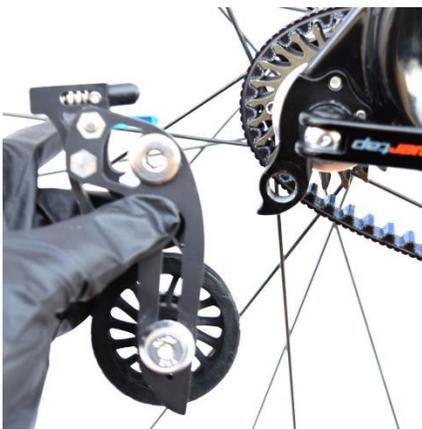
5. Start screwing in the titanium hanger bolt until the resistance drastically increases (torque spec). The tensioner arm should rotate about the bolt with a small amount of resistance and no play.
