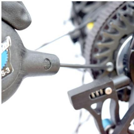
6. Next, rotate the tensioner arm upward until the idler wheel gently touches the belt.
