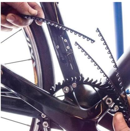
2. Bring the ends of the belt together so they form a “V” and align the teeth to each other. (Remember the belt should be looped around your chain stay)
