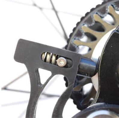
With the system preloaded in this manner, tighten the blue thumb screw to lock.
