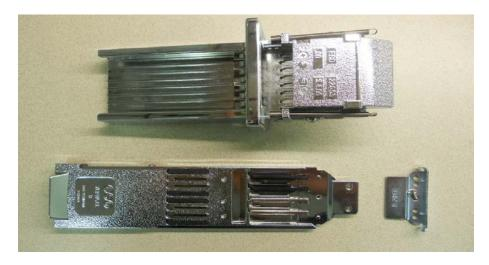
**Step 3:** Turn coin chute upside down and install or remove required number of plugs to change vent price.
