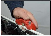
Pull the cutter along the length of the ski with firm downward pressure. If the cutter is
