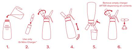
iSi Nitro Charger™ filled with Nitrogen Gas for use only with iSi Nitro Pro™
