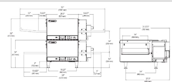
**Electrical Service:** Heat is supplied by one (1) element at 5600 watts. Each oven is rated at 6kW. The ovens are available in 208V and 240V and are single phase. The oven comes with a factory installed cord wth NEMA 6-50 plug. A separate circuit breaker is required for each oven deck with the proper voltage, amperage, phase and hertz as indicated by model number.
