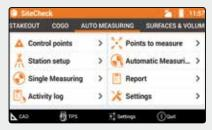
X•PAD Automeasuring is the simple, flexible, safe and economical solution for all you need to use the total station for automatic measurement and real-time checking of the movements of embankments, dams, buildings, bridges and other structures.
