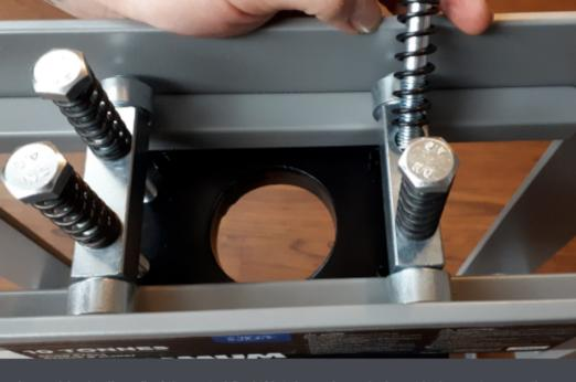
Assemble the 'head' of the unit. I find if I tighten these bolts with the springs until they just come out on the bottom of that black plate with the big hole, the tension is good on the rollers.
