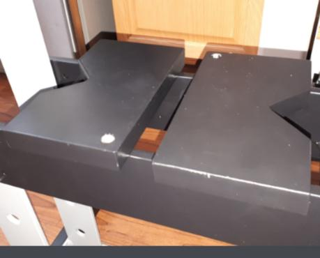
The 2 half plates that come with the press can be used with a bit of duct tape. Yup. You heard me. Duct tape.
