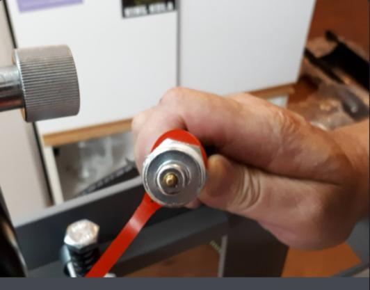
Inspect the pump hose end. Be sure it looks undamaged and be sure you dont have tape sitting on that flat surface Tape should only be on the threads. You can see the spin collar on the ram cylinder. When you tighten this get some paper towels and put it under the connection points throughout this assembly. Be prepared for minor oil loss when connecting joints.
