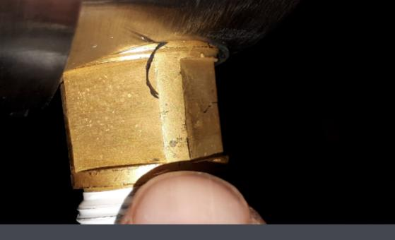
When attaching the gauge, do not use the gauge itself to tighten it to the press. See this brass fitting.. use a crescent wrench on this part to hold the gauge it the spot you want to view the face of the gauge.
