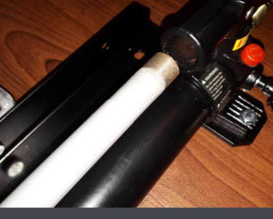
Attach the pump to the side of the press using the bolts supplied. Screw the handle into the pump.
