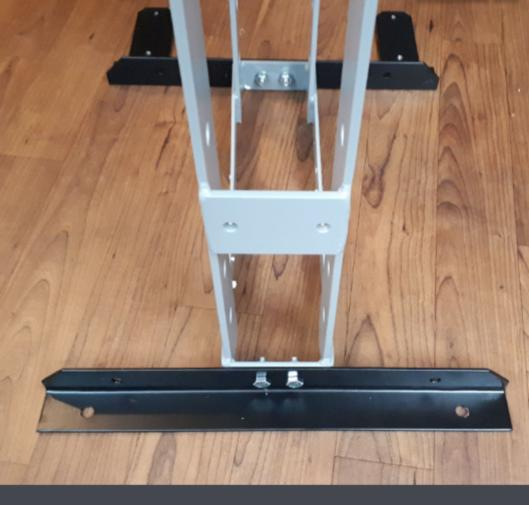
Here is the base assembled. If the frame wobbles in any way, (give it a shake!) then you need to get those nuts and bolts tighter!
