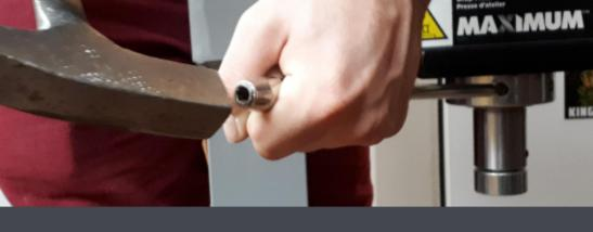
After positioning the ram, get a hammer and some kind of metal rod or a heavy duty screwdriver. You can see what I am doing in the picture above Hit this ring as many times as you have to UNTIL it stops moving.
