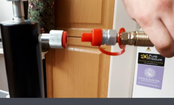
This is the joint for the pump hose. Take off these plastic protectors
