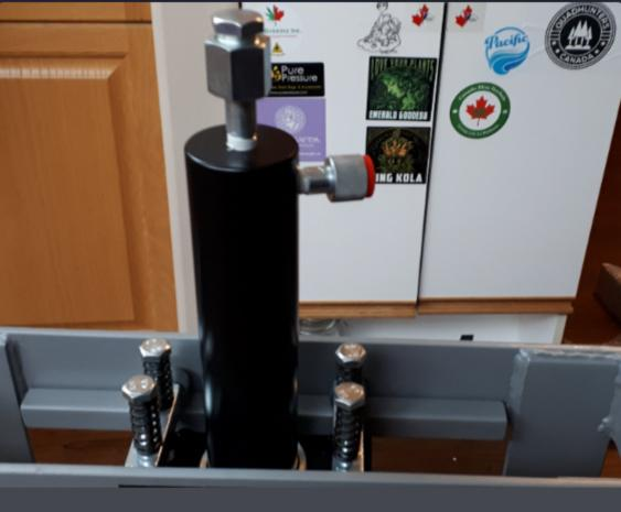
Here is the position of the ram outlets for RIGHT HANDED users. Spin it the other way for LEFT HANDED users! Have the one coming out the side pointing just a little bit to the back of the frame. This is where the hose of the pump attaches. Position accordingly. Go to next image.
