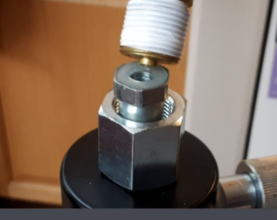
Ok now that the pump hose is attached, let's do the gauge. Apply plumbers tape again. So when you 1st get your press there will be a metal plug in here. Take that plug out (I have already removed it and the spin collar is loose.
