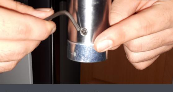
Now would be a good time to check and see if this piece is snug and not hanging/dangling down. If it is loose then hold it in place snug up to the ram and tighten this set screw with an Allen Key. You do not want this loose!
