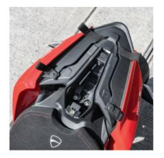
Slide an M5 washer inside each hypalon end of the 2 x bolt-on loops.
