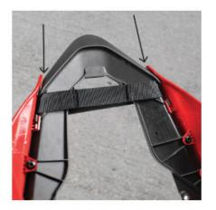
Locate the webbing between the inner and outer plastics, this maybe a tight fit. Once secured, then replace the rear cover.
