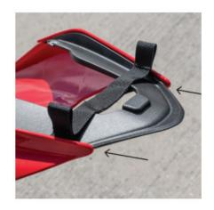
Remove the pillion seat, unscrew and remove the rear cover.
