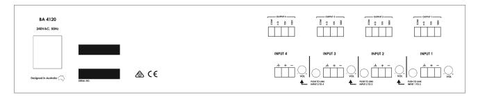
Mains Socket: The unit is connected to the mains circuit with a standard IEC type power lead. This socket contains a rated slow blow fuse.
