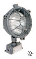
Designed for use on Merchant Vessels this Super Rugged fixture meets the requirements of the U.S. Coast Guard. Constructed of light weight, heavy-wall cast aluminum alloy with weather and saltwater resistant polyester powder coating. Stainless steel hardware used throughout. The lamp housing has a weatherproof clear lens cover which is mounted in a hinged guard. Three evenly spaced wing nut clamps secure the hinged guard against a resiliant sealing
