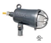
Constructed of light weight, heavy-wall cast aluminum alloy, with optional weather and salt water resistant polyester powder coating. Unit has patented spring mounted, porcelain mogul socket and heat resistant silicon rubber lamp sealing gasket providing maximum protection against shock, vibration and dust & moisture. Gasket compensates for lamp tolerance variation thus insuring snug fit. Flexible cable enters lamp housing through a water tight gland.
