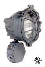
Circle-D's Heavy Duty Marine Light is designed with 3 equally spaced bosses (120° apart), blind tapped %"-16 for solidly shoring to bulkhead or structural member of merchant vessel. Intended to resist pounding of heavy seas. Constructed of light weight heavy cast aluminum alloy. Lamp housing has a weatherproof clear lens cover, mounted in a hinged ring. Three evenly spaced wing nut clamps secure lens ring against a resiliant sealing gasket, lamp housing interior and lamp are thus protected
