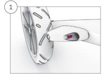
The brake should be adjusted if the brake force applied to the wheel is insufficient (this can occur if the tyres are worn) or the parking brake is difficult to activate (which is most often seen after replacement of a worn down tire). Always set the handle to the desired height before the brake is adjusted as the positon may cause a little variation of the brake adjustment.
