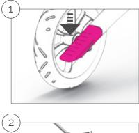
Even though Carbon Ultralight is the world's lightest walker and therefore is easier to lift, it is equipped with a kerb lifter that makes it easier to get over smaller obstacles like kerbs and low steps. This is particularly helpful if heavy objects are transported in a front-mounted basket or bag.
