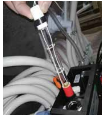
Step 5: Pull out the bulb to change it
