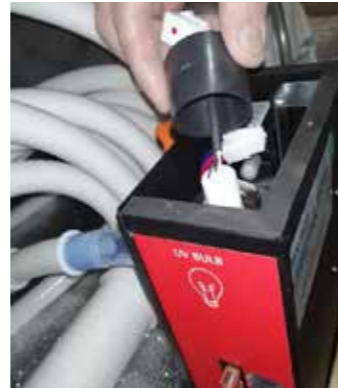
Step 4: Take out this black protective sleeve
