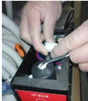
Step 7: Plug in the white connector
