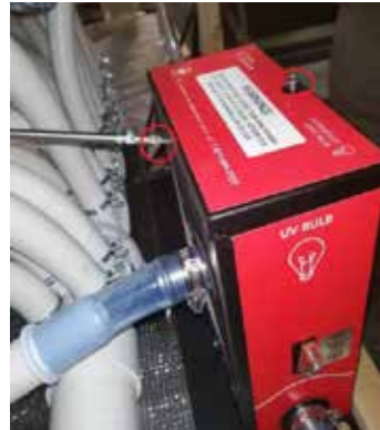
Step 1: Unscrew the 2 red-marked screws.
