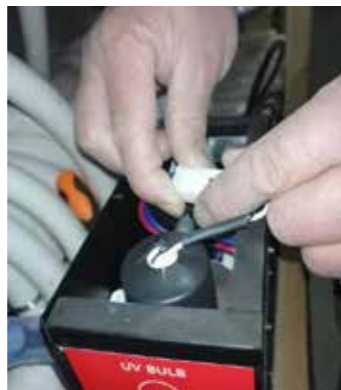
Step 7: Plug in the white connector
