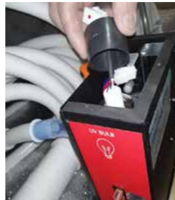
Step 4: Take out this black protective sleeve
