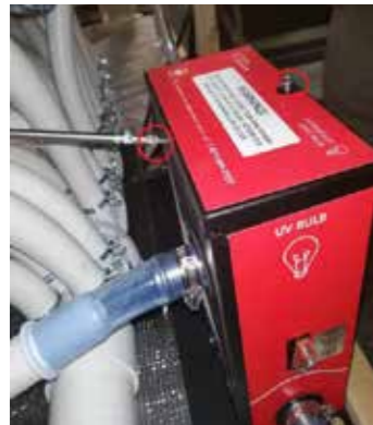
Step 1: Unscrew the 2 red-marked screws.
