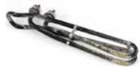
Low PH and low-quality chlorine causes the heater element to calcify
