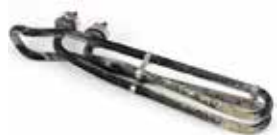
Low PH and low-quality chlorine causes the heater element to calcify
