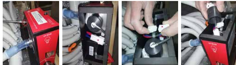
Step 1: Unscrew the 2 red-marked screws. Step 2: Remove the red lid Step 3: Unplug this white connector Step 4: Take out this black protective sleeve
