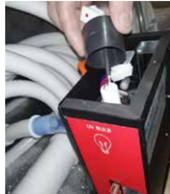
Step 4: Take out this black protective sleeve
