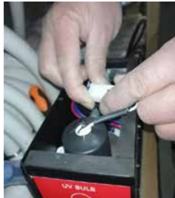
Step 7: Plug in the white connector
