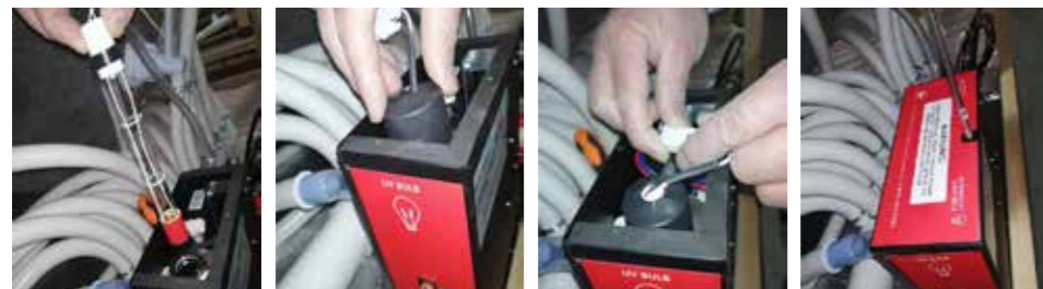
Step 5: Pull out the Lamp to change it Step 6: Put the Lamp inside the metal tube and cover it with black protective sleeve Step 7: Plug in the white connector Step 8: Cover the red lid and install these 2 screws
