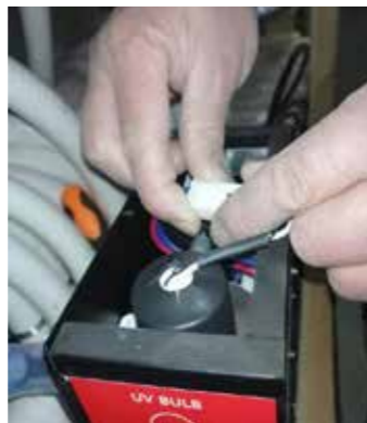
Step 7: Plug in the white connector
