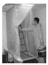
If desired, place ladder inside unit on base. Ensure ladder is stable prior to use. ABACUS unit will accept ladders up to 6' tall; TopSider unit will accept ladders up to 8' tall. Close all zippers and Velcro® seams.
