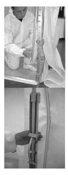
Step inside unit. Raise extension poles by lifting one or two notches at a time, alternating sides until unit is at desired height. For best results, unit should be fully extended. Slide down locking collar.
