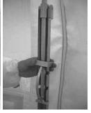
Step inside unit. Raise extension poles by lifting one or two notches at a time, alternating sides until unit is at desired height. For best results, unit should be fully extended. Slide down locking collar.
