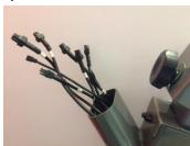
(NOTE: IN SOME UNITS, A PLASTIC TIE WILL SECURE THE CABLES IN THE SPINE. IF IT IS PRESENT ON YOUR UNIT, CUT THE TIE PRIOR TO ROUTING THE CABLES UP THROUGH THE TOP OF THE SPINE. BE CAREFUL AND DO NOT CUT THE CABLES)
