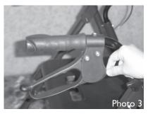
3. To adjust the position of the brake pad, rotate the metal nut in front of the brake handle. [Photo 3]
