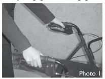
1. Applying brakes: Squeeze both brake handles to slow or stop. [Photo 1]
