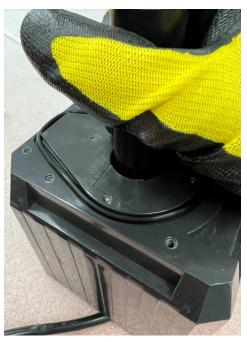
Wipe all surfaces down with 99% Isopropyl Alcohol. Pull the ceramic shaft out and use a q-Tip or pipe cleaner to scrub out the skinny sections. Clean the ceramic shaft along with every nook and cranny.
