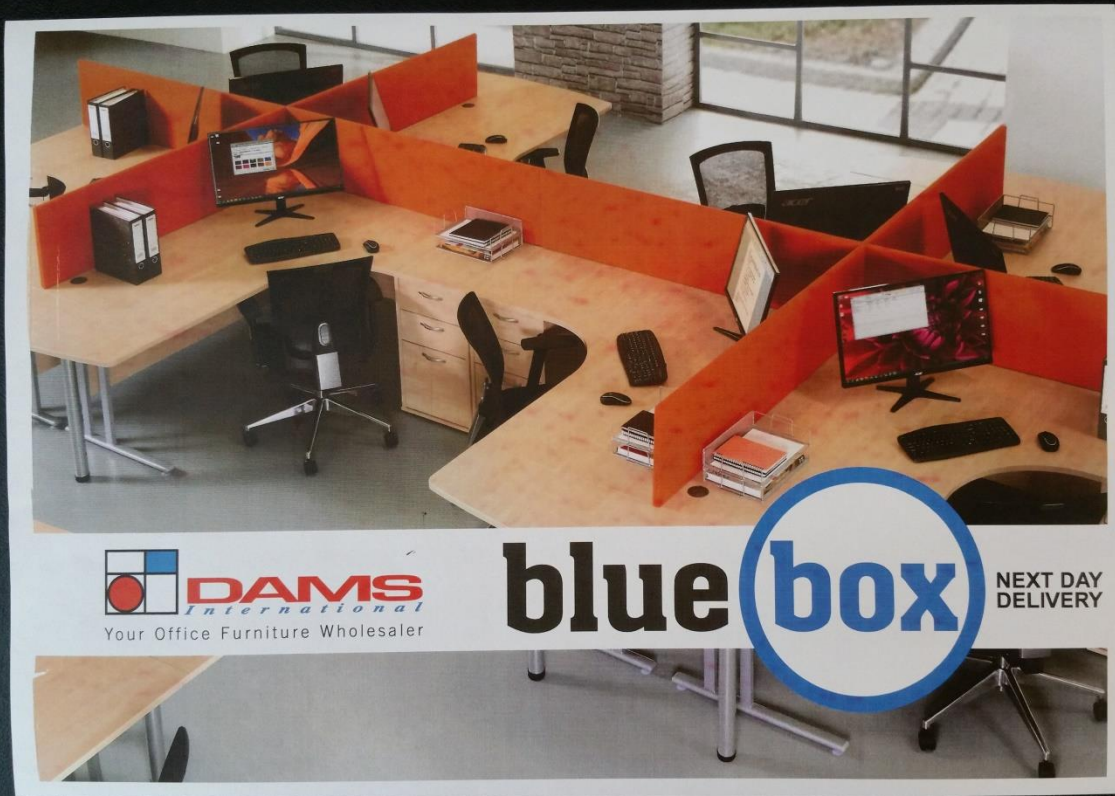
Photocopy produced on an OKI MC851 using compatible Toners sourced from the largest Toner supplier in the UK, note mottled background on desk tops and desktop screens.
