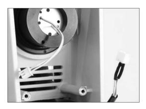
• Loosen LED board locating ring, take away LED board locating ring.
