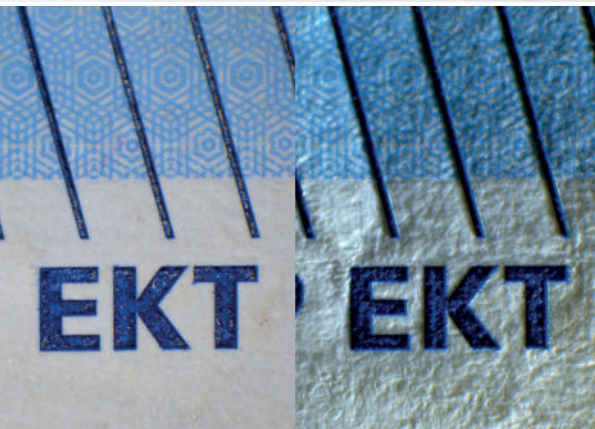
€20 banknote: Ring light illumination / horizontal illumination
