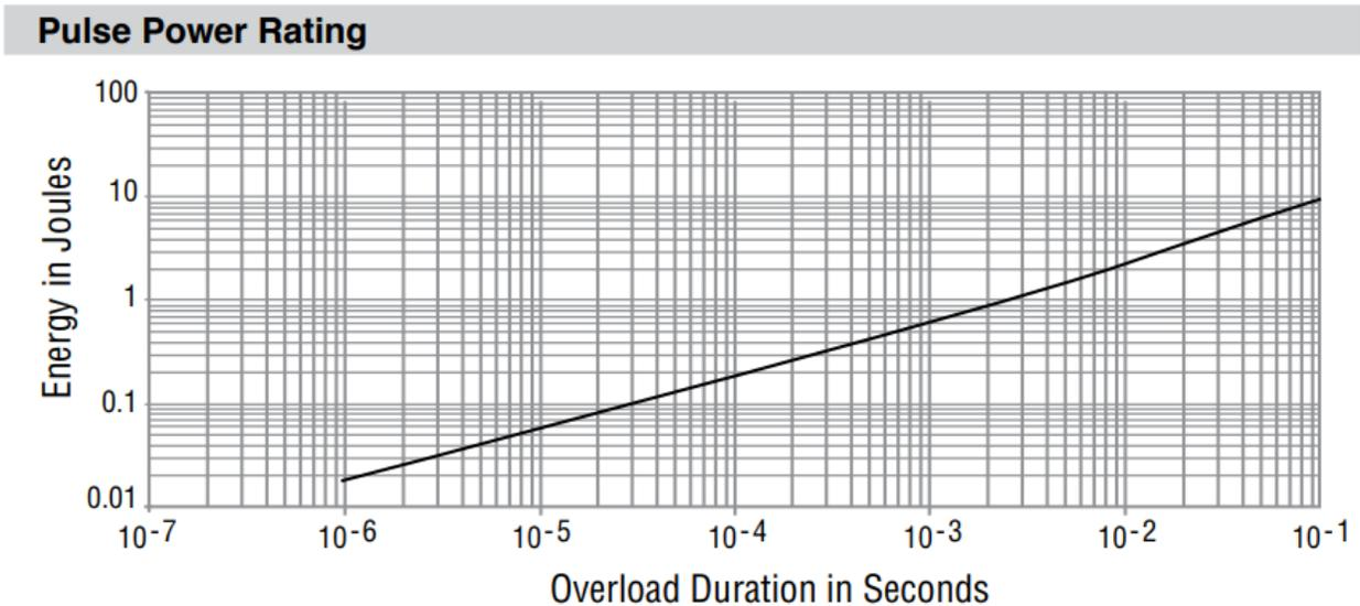
For 1 second, the spec has prescribed 25J (25W \* 1sec @ 25C). For 100 mS, we see a single load resistor can handle 10J of energy. Note that 1J = 1W for 1 second, and thus 10J = 100W for 100 mS. So, the array of 8 resistors (when configured as a 4 ohm load) can handle 800W for 100 mS. If using as an 8 ohm load, this figure is 400W for 100 mS.
