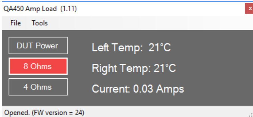
Pressing an illuminated load button again will turn the loads off. When both the 4 and 8 ohm buttons are off, then the QA450 presents an “infinite” or open load to the amplifier. Note that when the QA450 is open, the QA450 +/- outputs are meaningless. That is, the input signals cannot be measured when the loads are disconnected.
