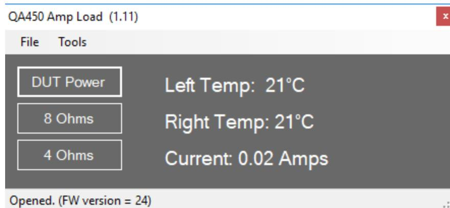
In the title bar, you can see the version of the software, shown here as 1.11. In the status bar, we can see the hardware device is "opened" and that this is firmware version 24. You will be alerted if the firmware version is incorrect and given a chance to re-flash the QA450 hardware. It is important to NOT use the application if the firmware version is reported as incorrect as malfunctions could occur.
