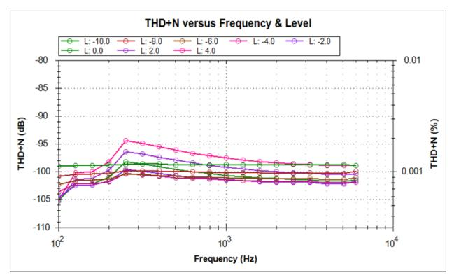
The plot below shows the THD+N ratio with the output swept from -48 to 4 dBV.
