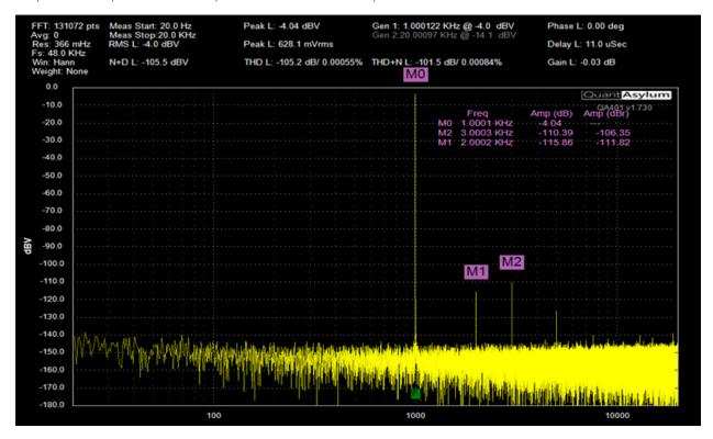
The plot below shows the achieved THD+N at level swept from 100 to 6 kHz and from -22 dBV to -6 dBV. The harmonic measurement limit was 20 kHz.
