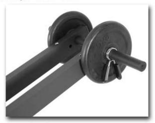
Add the larger weights first followed by smaller weights. When the proper amount of counterweight has been added, the crane will rest in a horizontal position Motion will be smooth and effortless. Once the crane is balanced, secure the weights by adding the clamps to the outside as shown above.
