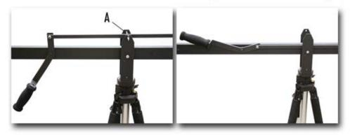
Below, the camera is manually tilted downward on the overslung camera mount. <a href="MARNING"><u>WARNING</u></a>: When tilting manually, ALWAYS maintain control of the camera. A front heavy camera may rotate forward abruptly and without notice.
