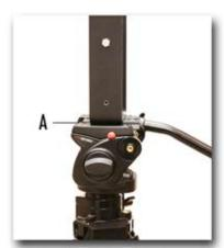
With the stand mount attached to the crane, set it on top of the stand's main shaft. Tighten the knob (A). To raise the shaft, loosen knob (B), raise shaft, insert pin (C).
