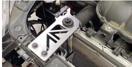
3. Using the supplied 1/2"-20 hardware, attach the catch can(AOS) to the stainless mounting bracket with a 5/32" Allen Wrench an 7/16" Wrench
