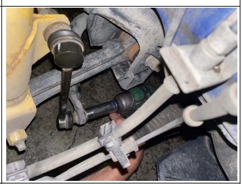
4.5 Set aside OEM endlink and hardware, new hardware is supplied.
