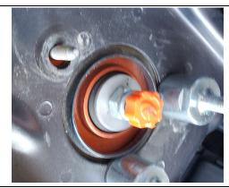
top of each stud and screw the standoffs down to the shock tower studs. You can use a 1 ½ crows foot and torque them down to 20 ft lbs or 239 in lbs. If the crows foot is unavailable you can use an adjustable wrench. If using adjustable wrench DO NOT over tighten or you risk breaking the stud.
