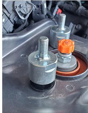
Place the assembled base plates on top of the standoffs. Put the 15mm nuts on top of the standoff stud.
