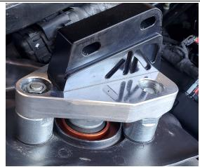
over the riser plates, and insert the 4 M8x60mm bolts through the holes in each end. Note: Because the shocks have some play within the shock towers. Some bolts might be harder to line up, leaving all bolts loose will help generally but you may have to force the last one through.
