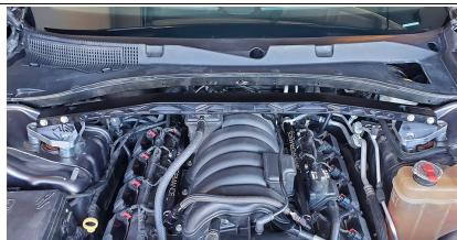
6. Tighten the(6) 15mm nuts on the base plates to 25-30 ft lbs and tap your dust cap over the holes using a rubber mallet. Then tighten the (4) M8 bolts to 17 ft lbs using the 13mm socket and wrench.
