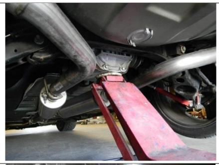
5B. Using an air saw or Sawzall, cut a small notch in the sheet metal that obstructs access to the Upper Tension Arm chassis-side retaining bolt. Loosen the retaining bolt enough to allow a saw blade to reach the bolt, then use the saw to cut the head off of the OEM bolt and remove it. It is recommended to use lubrication such as WD-40 during cutting. Perform this step for each side of the vehicle.
