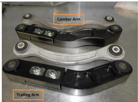
4. Work on one side of the vehicle at a time. First, removing the OEM Control Arm (arm near the shock) using the 18mm wrenches and replacing it with the AAD Performance Adjustable Control Arm.
