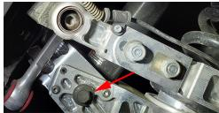
3. Pull back the inner fender liner and remove the 10mm bolt holding the brake line bracket. On the drivers side only.
