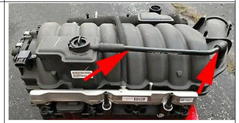
3. Locate and remove the upper 15mm stud and 13mm bolt from the front timing/water pump housing.
