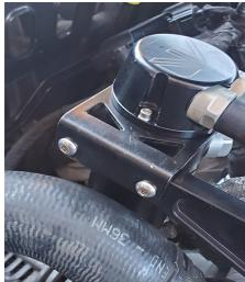
7. Insert hose from PCV valve to the bottom barb fitting on the can. Insert hose from intake side to the barb fitting on the top of the can. Note: if you purchased the ½ to ½ barb fitting insert into the factory rubber connection. If you didn't connect the hose directly to the factory nipples on the manifold.
