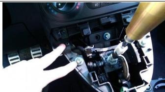
**Step 6:** Remove the screws as shown in the attached pictures to remove the console trim panel
