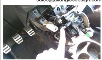
**Step 9:** Remove the new AAD Short Shifter from the box and locate the Shift Arm. Using the two provided Socket-Head Cap Screws, assemble the Shift Arm to the rest of the shifter with the small detent facing the rear of the vehicle. This detent aligns with the notch in the shift knob to keep the knob properly aligned. Make the two SHCS snug, but do not over-tighten.
