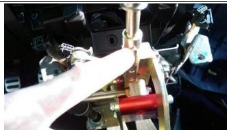
**Step 10:** Slide the shift cables back in place on each side of the new AAD shifter and re-install the cable retainer clips – reverse of Step 8
