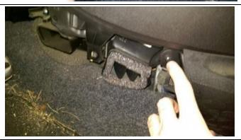
**Step 7:** Remove 3 nuts and 1 bolt holding the stock shifter onto the dash frame
