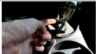
**Step 8:** Remove the two shift cable retainers and remove the cables from the shifter. *NOTE: You can reverse the order of steps 7 and 8 if you wish, but removing the shifter from the chassis first affords more space to get at the cable retainers.*
