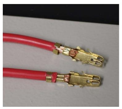
Figure 3: A bad crimp (TOP) has too much insulation stripped, poorly crimped wire holders and the insulation holders are smashing the little bit of insulation they are touching. The crimp on the bottom is 100% reliable.
