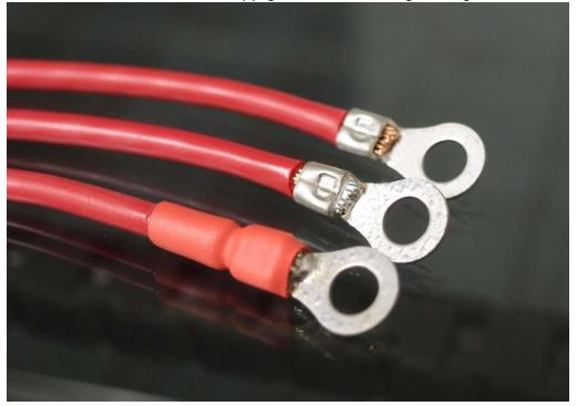
Figure 4: A proper soldered joint is first crimped (TOP), then soldered with good flow (MIDDLE), then protected with double-wall heat-shrink tubing (BOTTOM).
